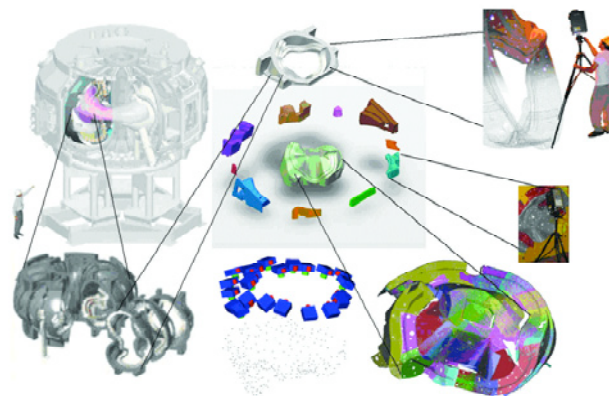
Figure 3: Digital assembly techniques made it possible to scan and assemble this large 40-plus part assembly of patterns used to cast a fusion reaction chamber. This technique determines how the complex cores assemble together to define final casting dimensions.
