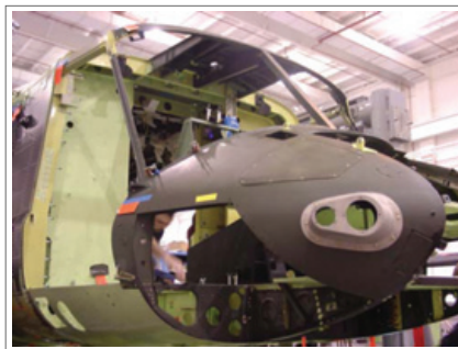
ASSEMBLY VIA TEMPLATES
