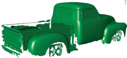
STL POLYMESH USED AS A BASIS FOR REVERSE ENGINEERING.
